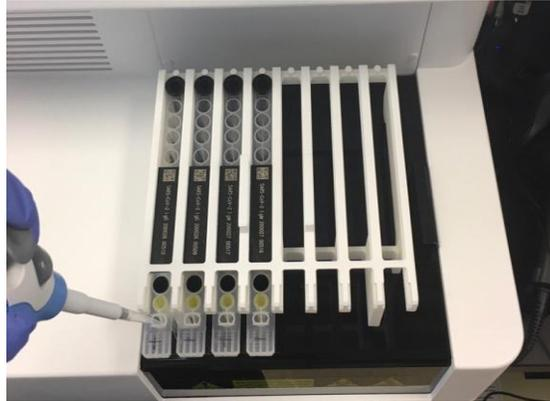
*Figure 4: Adding Controls to the Cartridge*
