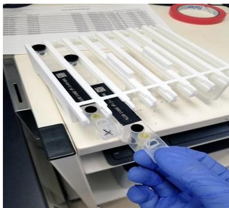
*Figure 3: Inserting Controls Cartridges into Reagent Rack*
